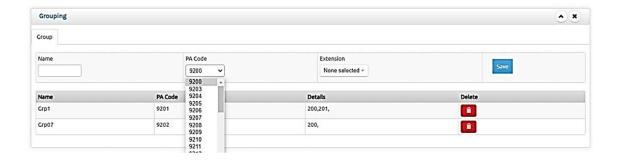
In Traditional paging systems, zone creation is done via hardware and is very complicated with a limit on the number of zones. Whereas with our SIP paging 100 differed zones can be created with various sets of speakers. In addition individual speakers can also be accessed by dialing their respective extn nos.
